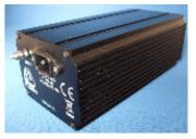
LNB Supply: Two LNB power supply outputs on a 9-way D-type socket. Maximum current 500mA per output. Factory set to 18V d.c. (Other voltages on request). Thermal and overcurrent protection. Output voltage and current available through the serial port.
